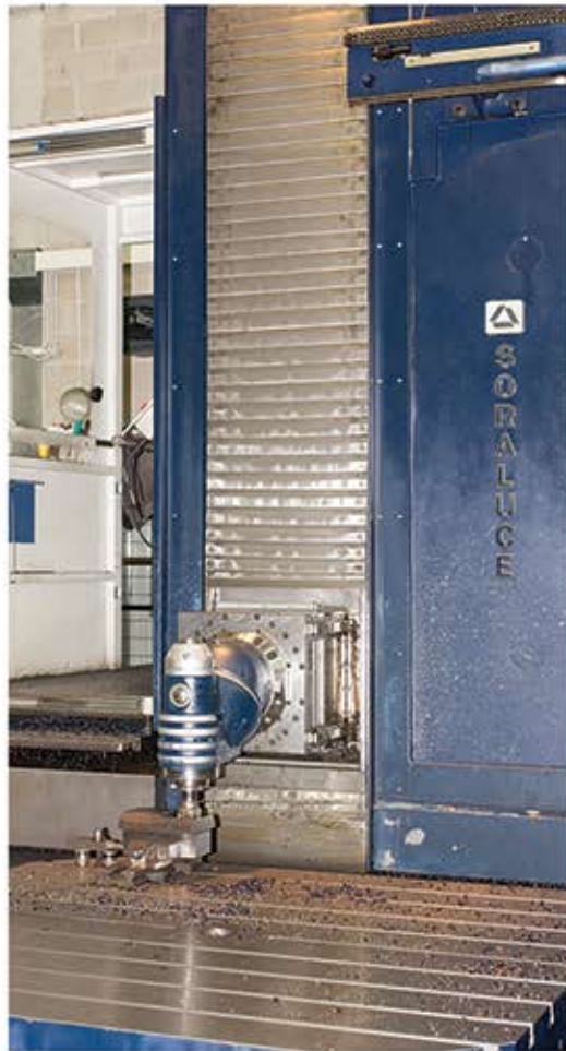
1 FL8000 model with a SORALUCE universal head
